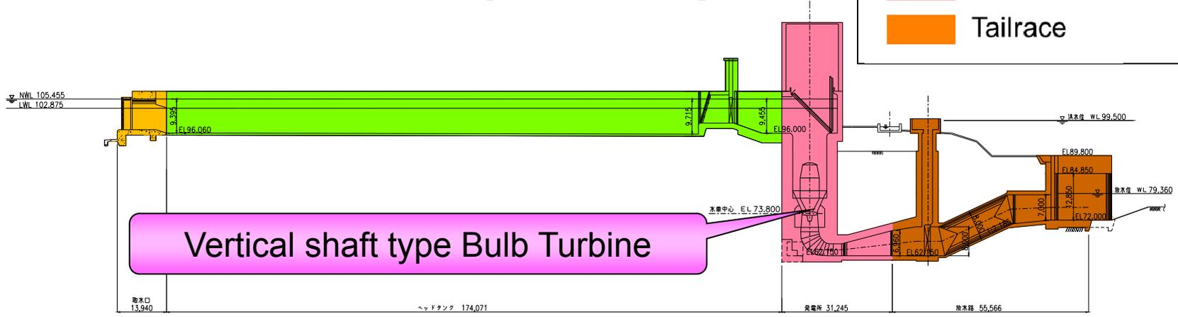
Vertical shaft type Bulb Turbine
